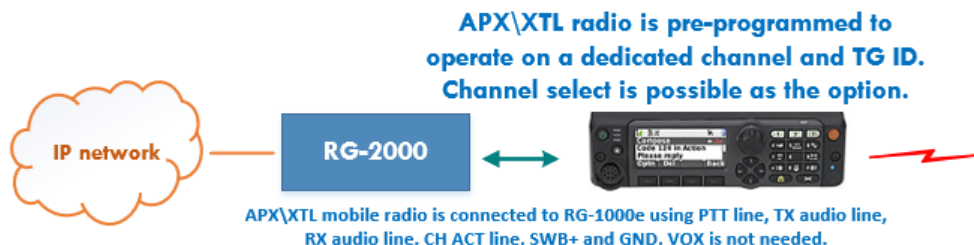
Fig. 4 Motorola APX\XTL radio connection to RG-2000
