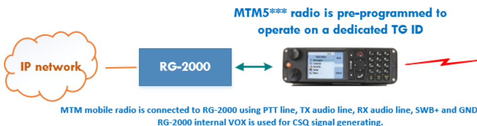
Fig. 5 Motorola MTM radio connection to RG-2000
