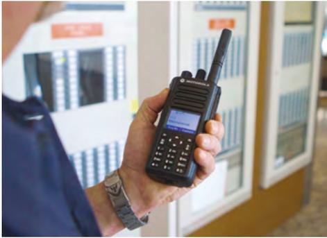
The Motorola Indoor Tracking solution requires the Enhanced MOTOTRBO radios (i.e. XPR7550e/ DGP™ 8550e / XiR P8668e/ DP4801e). The radios should be Bluetooth equipped and Indoor Tracking support should be enabled. These radios can then communicate with any Bluetooth Beacons that support the iBeacon protocol (i.e. Estimote or XY Find It).
