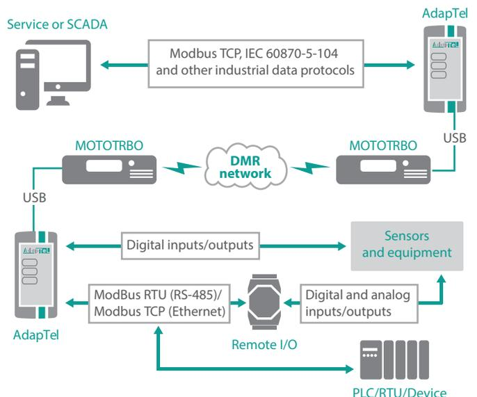
AdapTel collects technological signals and controls technological equipment through built-in digital input (DI) and digital output (DO) channels, as well as through third-party input/output expansion modules using Modbus data protocol.
