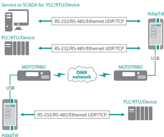
AdapTel provides transparent channel for communication between third-party devices (PLC/RTU/Meters/Sensors/etc) and SCADA software in DMR network.
