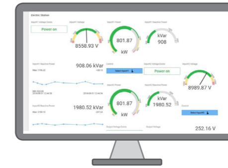
Real-time equipment monitoring using a set of widgets (gauges, bars, indicators, boards, graphs and so on)
