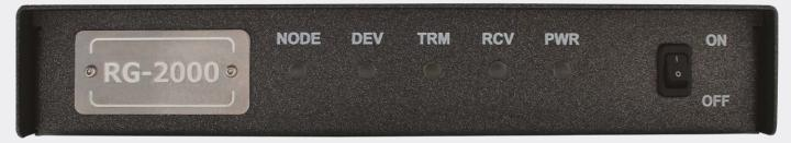
RoIP gateway to connect remote donor radios such as MOTOTRBO, P25, Tetra, and analog to the SmartPTT radioserver for interoperability
